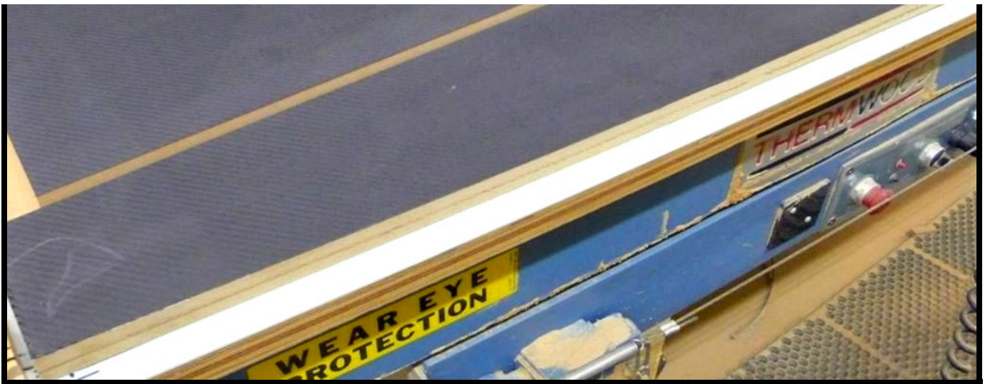
A CNC router cuts Model Seven body panels from constrained-layer-damped composite material -- a nine-layer sandwich formed from several grades of carbon fiber, HDF, and an elastomeric membrane.
