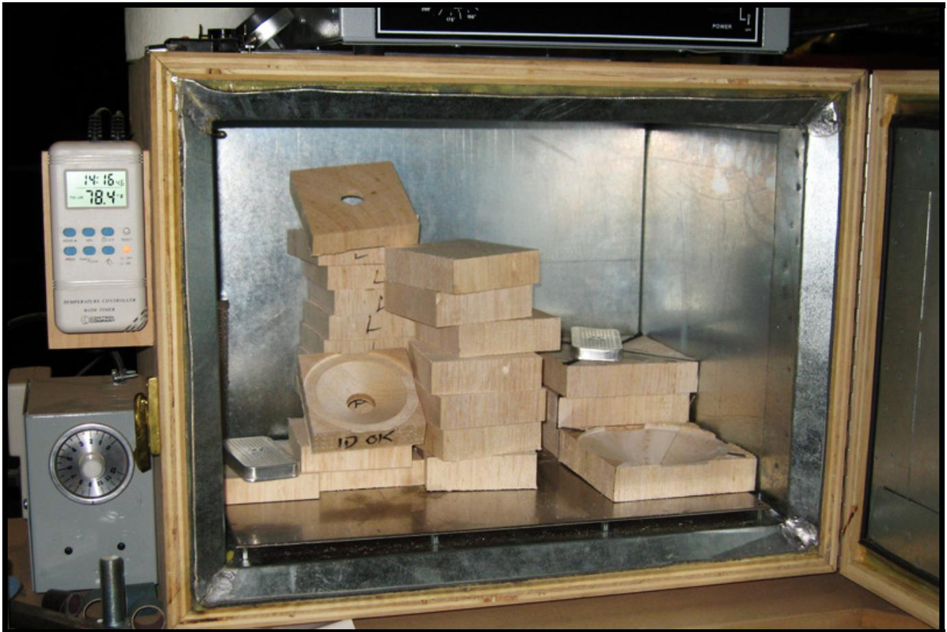
**Balsa cut into 4" x 4" x 1.25" blocks, from which the driver cones are machined, "baking" in a special oven to remove all residual moisture -- a necessary step to ensure proper lamination of the cone skins of ultra-high-modulus carbon fiber.**
