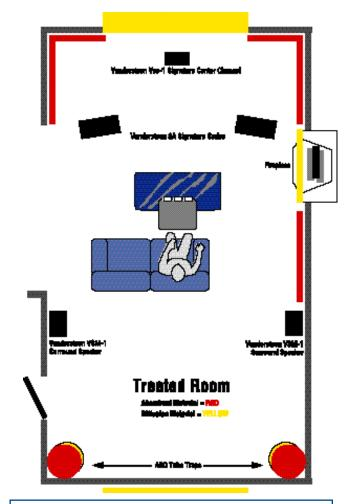
Reflections coming from surfaces near the speakers can confuse the ear and I like to place absorptive material beside and behind the speakers. In this room there is a bay window between the speakers and I covered that with wide-blade, plantation shutters which act as sound diffusers for stereo listening, and block most of the light for home theater viewing. Shutters also cover the window at the rear of the room.
