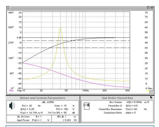
This illustration shows the amplitude and phase characteristics of a sealed enclosure subwoofer with a Qtc of 0.5, at frequencies below system resonance which, in this example, is 40Hz.
