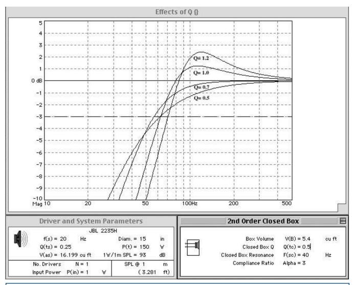
This illustration shows the effect of system Q on frequency response. Notice that the low-Q alignments start sloping down sooner but ultimately extend lower in frequency at the usable low frequency limit of -10dB. Remember that the low-Q alignments provide far better damping to oscillation after the signal ceases.
