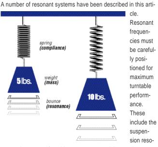
nance, the tonearm/cartridge resonance, and the cantilever resonance.
