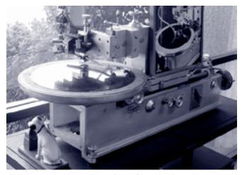
the lacquer coating on the surface of the aluminum master disc. A vinyl record is produced from this master disc (several intermediate stages are involved). During playback, the pickup cartridge converts the groove wiggles into an electrical signal that can be amplified and reproduced as sound.
