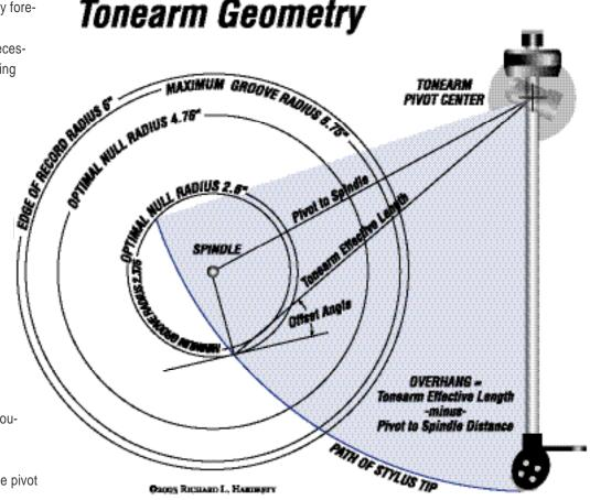
when geometry is adjusted correctly. Proper geometry requires optimum offset angle and stylus overhang.
