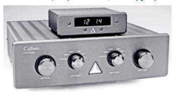
Aesthetix sent over the top-of-the-line \$14K Callisto Signature tube line stage, which is a purist design to the extreme. It's a three-box design, with a separate power supply, separate input selector, and separate volume control for each channel. And that doesn't include a remote control, which is a \$2,000 option.
